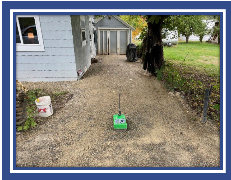
Looking South. Completion of nuclear density testing. Image provided by CDA Trust.
