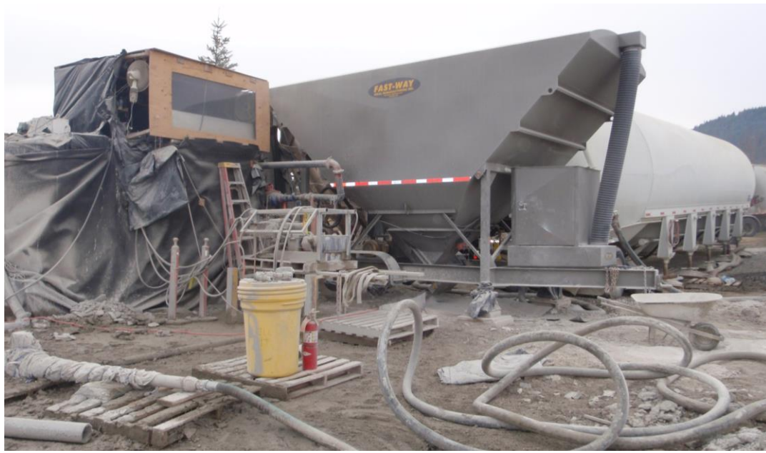
Concrete Batch Plant Set-Up
