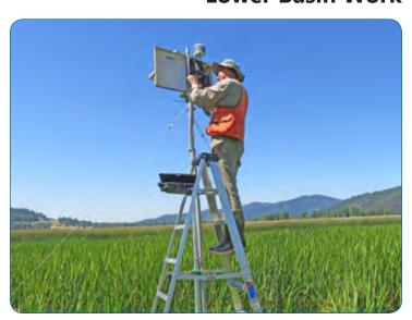
EPA's Office of Research and Development recently installed two data stations in Lane Marsh, in the lower Coeur d'Alene River Basin. The stations are collecting important environmental data to inform research on in-place methods to clean up lead in marsh sediments.
