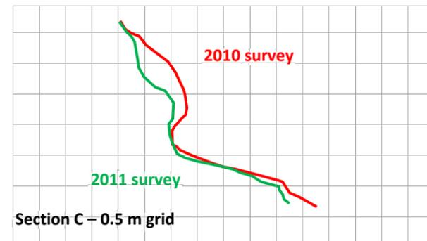
Exhibit 19. Terrestrial Laser Scanning Example Bank Analysis, Medimont Scanning Location
